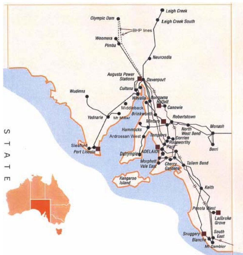
ElectraNet's transmission network
